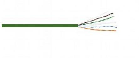
Kramer's BCLS-21 is a high-performance CAT 6 U/UTP cable designed for IT, LAN and Ethernet installations. It is constructed with four pairs of 23AWG solid bare copper conductors with a cross filler. It is enclosed in an LSZH jacket with internal rip cord and sequential markings every meter and packed in a Reelex II carton for easy to pull-out. BCLS-21 cable exceeds CAT 6 specifications to provide additional performance and bandwidth beyond the basic standard
